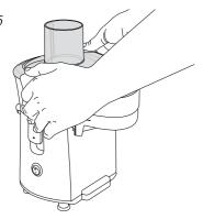
6. Slightly tilt the pulp container and slide into place under the juicer cover.
